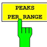
The *PEAKS PER RANGE* softkey defines how many peaks are searched for within one range. The ranges are according to the band class setting (SETTINGS -> BAND CLASS) e.g. for BAND CLASS 0, 2, 3, 5, 9, 10, 11 and 12:
