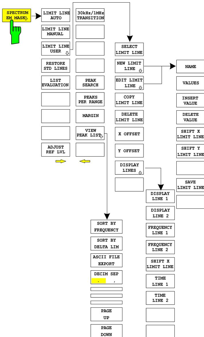
The *SPECTRUM EM MASK* (Spectrum Emission Mask) softkey measures the signal power in defined offsets from the carrier and compares the power values with the spurious emission mask, specified in the cdma2000 specification, in the near-carrier range from -4 MHz to 4 MHz.
