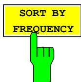
The *SORT BY FREQUENCY* softkey sorts the list in ascending order according to the column *FREQUENCY*.
