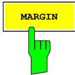
The *MARGIN* softkey defines an overall margin which is subtracted from the limit line to make the peak search more stronger. If the values of the trace are above the limit line minus margin value it will be marked with a cross as shown in the peak list. The DELTA LIMIT of the list will be positive thus indicating that only the margin and not the limit itself is reached. A negative sign would indicate the real fail. The default value of *MARGIN* is 6 dB.
