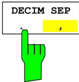
Different language versions of evaluation programs may require a different handling of the decimal point. It is therefore possible to select between default separators '.' (decimal point) and ',' (comma) using softkey *DECIM SEP*.
