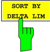
The *SORT BY DELTA LIM* softkey sorts the list in descending order according to the column DELTA LIMIT.
